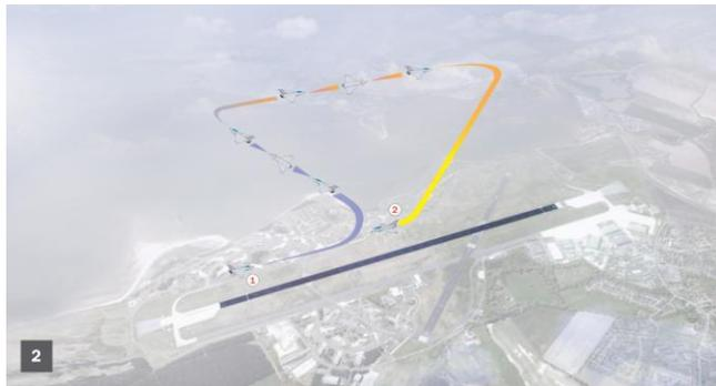
**2.** Just prior to datum the aircraft is turned hard at 9Gz away from the ground and after a roll and further turn the aircraft is positioned for the slow pass. Having passed the crowd at over 450 mph moments earlier the aircraft is now flying at less than 100 mph.
