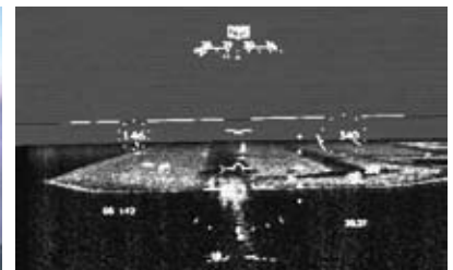
Even in dense fog, AALC allows the pilot to see the runway image for landing.
