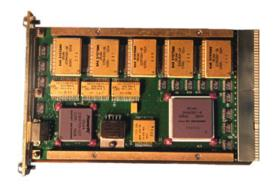
The 3U CompactPCI standard single-board computer, available in flight and prototype versions, employs the PowerPC RAD750® microprocessor, the radiationhardened version of the IBM PowerPC750. The companion PowerPC bridge ASIC provides access to the memory and the PCI version 2.2 backplane bus.
