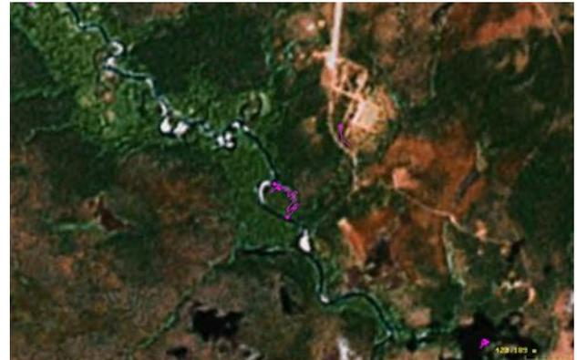
Fig. 8: Estimated group track position obtained from the data shown in Fig. 6. The correct group size, 3, was obtained. There are a couple of false tracks.
