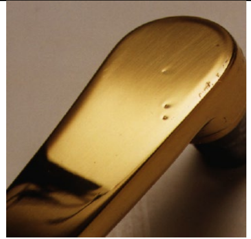
Figure 6. Example of large pinholes on a finished surface
