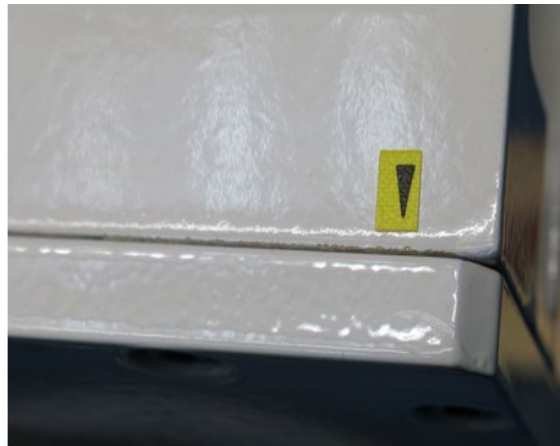
Figure 4-23 – Tape line chipping
