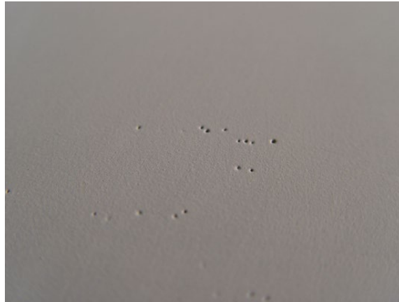
Figure 4-22 – Pinholes (Image demonstrates appearance only, scale unknown)
