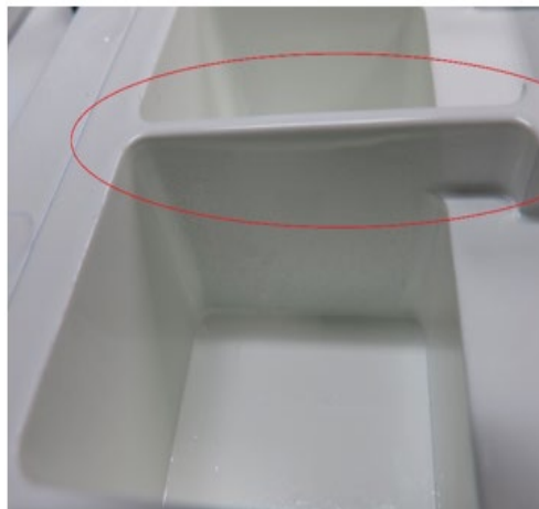
Figure 4-115 – Edge buildup - Minor paint buildup on edge, corners and appear to be rounded (not sharp) is acceptable
