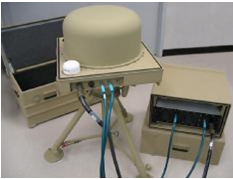
Antenna mounted on telescoping tripod
