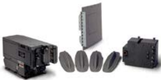
The AN/APX-113(V), AN/APX-125(V), and AN/APX-126 CIT systems have identical form factors
