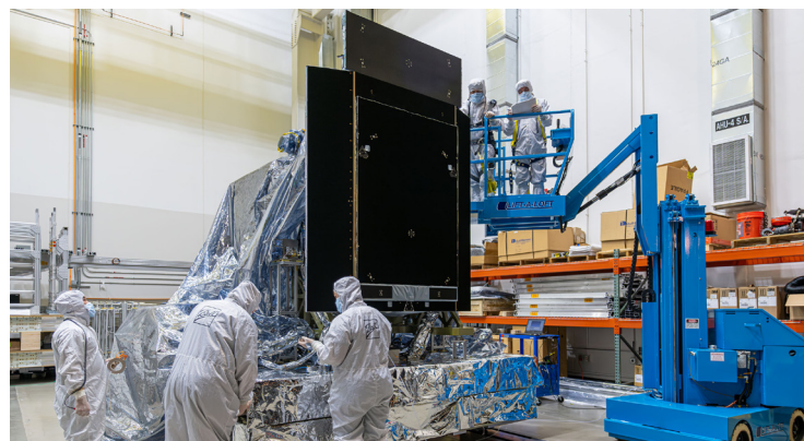
WFI radiators installed – prior to Thermal Vacuum Chamber (TVAC) testing
