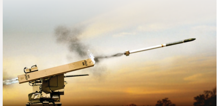
An APKWS laser-guidance system is utilized during a ground-based containerized weapon test fire.
