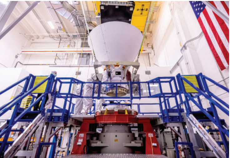
Spectro-Photometer for the History of the Universe, Epoch of Reionization and Ices Explorer (SPHEREx) on the vibration table
