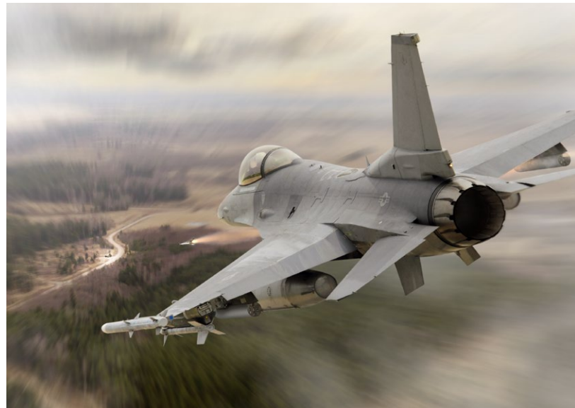
The APKWS laser-guidance kit is successfully operating in combat on the F-16, A-10, AV-8B , and several other fixed-wing platforms, as well as a number of rotary-wing platforms.
