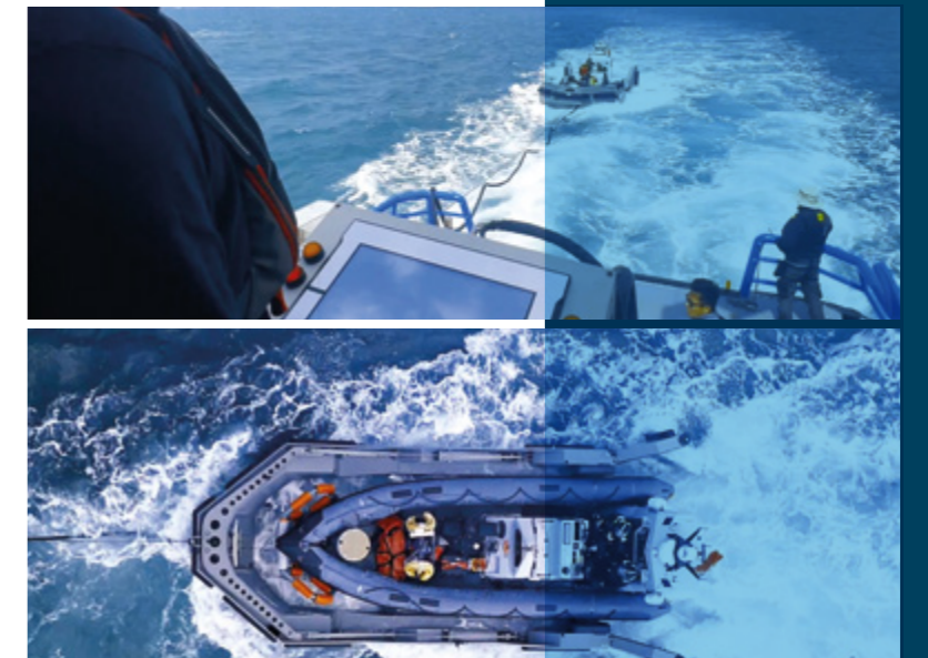
The autonomous launch and recovery system in action.
