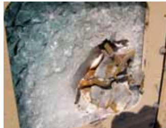
HMMWV window hit by IED – exterior and interior
