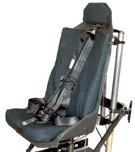
Cockpit seat with monolithic bucket
